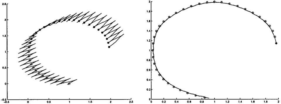
Figure 2: Stratified motion planning for hexapod robot: *i*) constant orientation,  $\theta = \frac{\pi}{3}$  radian (left); *ii*) tangent orientation; “o”: reference points, “+”: reached points (right)
