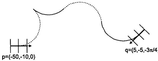
Figure 3: Trajectory along arcs of circles
