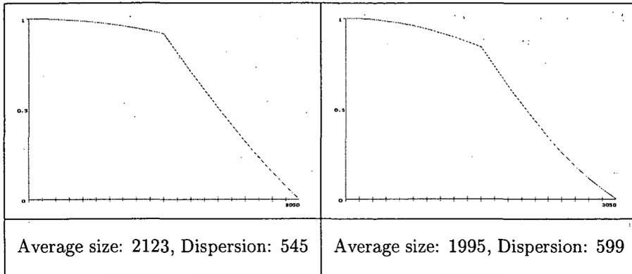
Figs 3-4. The oversize distributions of the particulate product at the outlet of the mill after  $t=10$ ,  $t=20$  units of time, respectively. Continuous grinding without recirculation. Discrete model number I. Parameters:  $I=20$ ,  $J=20$ ,  $m=2$ ,  $n=2$ ,  $V_F=0.5$ ,  $V_B=0.1$ ,  $L_{max}=3050$ ,  $K_s=9 \cdot 10^{-9}$ ,  $d=4$ .
