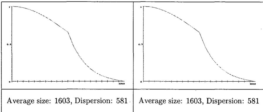
Figs 11-12. The oversized distributions shown at the outlet of the mill after  $t=1143$  and  $t=1153$  units of time, respectively. Continuous grinding with recirculation.
