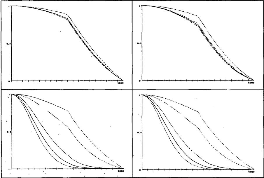
Figs 13-16. The oversize distribution functions shown in the first, third, tenth, fifteenth and twentieth columns of the mill at  $t=5^{th}$ ,  $t=8^{th}$ ,  $t=150^{th}$  and  $t=287^{th}$  units of simulation time. Continuous grinding with recirculation. Discrete model number I. Parameters:  $I=20$ ,  $J=20$ ,  $m=2$ ,  $n=2$ ,  $V_F=0.3$ ,  $V_B=0.1$ ,  $L_{max}=5000$ ,  $K_s=10^{-8}$ ,  $d=4$ .
