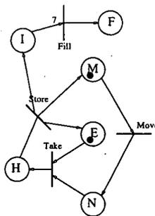
Figure 4: The Petri net with an initial marking for the box filling example.
