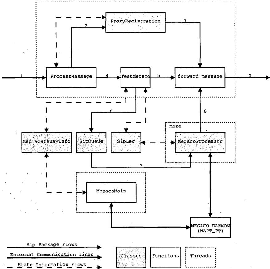
Figure 4: The functionality of SIP proxy on IPv6
