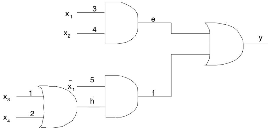
Figure 3: A single fault in a combinational circuit
