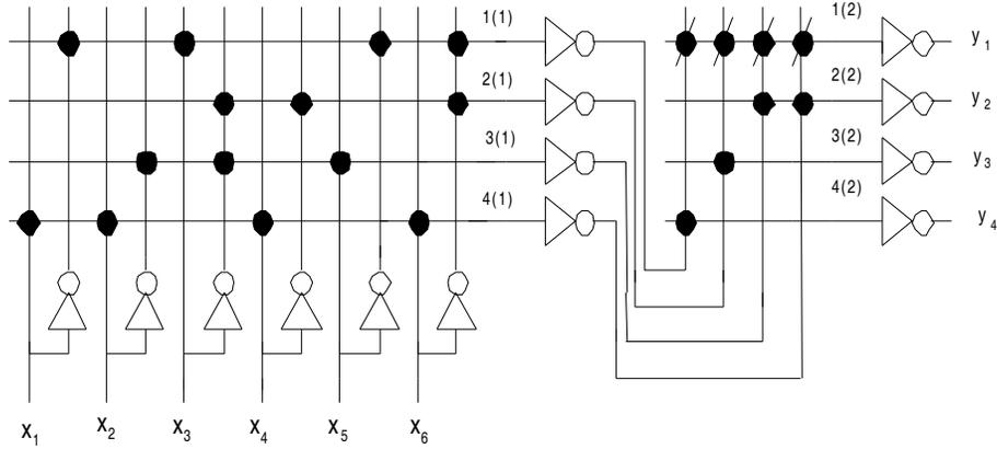
Figure 6: A multiple fault in programmable logic array
