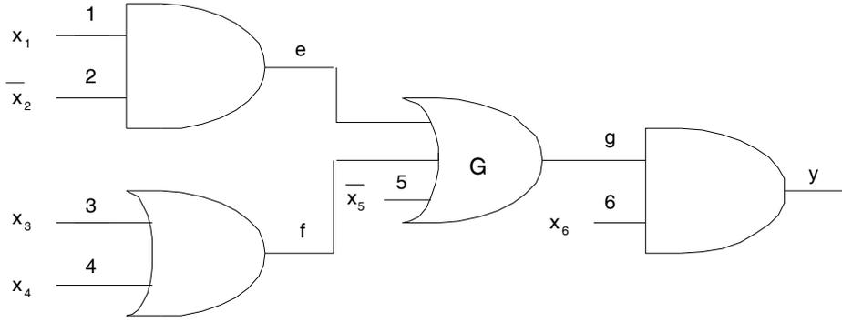
Figure 4: A double fault in a combinational circuit
