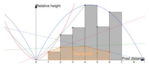
Figure 2: Distance–maximum height histogram for a given texel. The orange points are the height differences divided by the distance. The blue, red, and green lines form a convex boundary, and each line corresponds to a bounding parabola.
