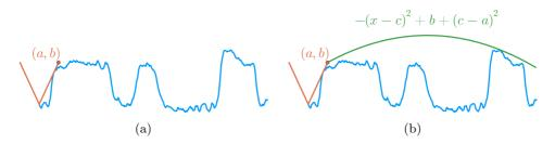
Figure 5: The two parts of generation of parabolas. First, we find values a and b, which define a cone (orange). Then, we calculate a parabola from (a, b) above the heightfield, defining an additional c parameter (green).
