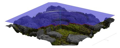
Figure 4: Generated radial function  $m_{uv}$  (red line) for a heightfield around the axis of the current texel (blue line). The value of the function at a given distance from (u, v) is the maximum height of the texels with the same distance.
