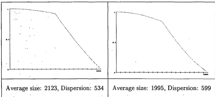
Figs 1-2. The oversize distributions of the particulate product at the outlet of the mill after  $t=10, t=20$  units of time, respectively. Continuous grinding without recirculation. Discrete model number I. Parameters:  $I=20, J=20, m=2, n=2, V_F=0.5, V_B=0.1, L_{max}=3050, K_s=9 \cdot 10^{-9}$ .
