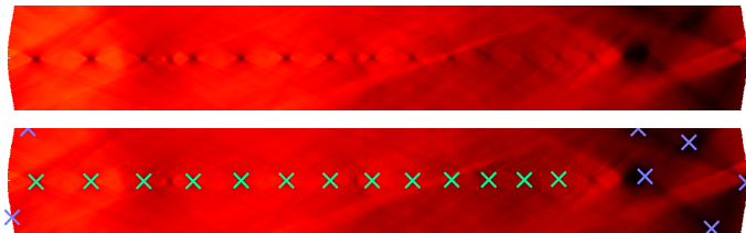
Figure 3: Example visualization of C cost function for horizontal wires. Horizontal axis is \rho and vertical axis is \theta . Brighter color means higher function value. Top: Negative peaks can be seen as dark spots. Bottom: All candidates as described in Section 2.3, filtered as in Section 2.4. Inliers are marked with green, outliers are marked with blue.
