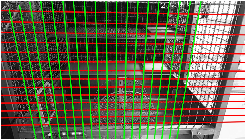
Figure 4: Found lines painted over the original image, vertical lines in green and horizontal lines in red.
