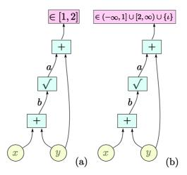
Figure 7: AST for the constraint  $y + \sqrt{x+y} \in [1,2]$  (left) and its complementary (right)
