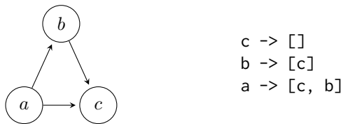
Figure 4: An example for dependent modules (Left). RefactorErl’s textual representation of the dependencies (Right).
